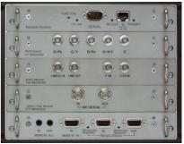
Two sets of terminal boards (network and remote control) are suppled. Up to three optional boads can be installed.
