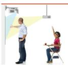
Ultra short throw creates a 77" standard or 87' widescreen diagonal image from a mere 23 inches. eliminating shadows on the screen along with projected light in the presenter's eyes created by traditional front projection systems.
