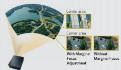
The Marginal Focus feature helps to ensure that images projected onto a spherically domed surface are kept in focus right up to the very edges.
