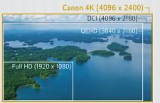
At 4096 x 2400, Canon's 4K resolution generates a bigger, richer picture made up of more than 9.8 million pixels – higher than the Digital Cinema Initiative (DCI) standard for 4K cinema (4096 x 2160) and more than QFHD (3840 x 2160), the resolution standard for 4K TV.
